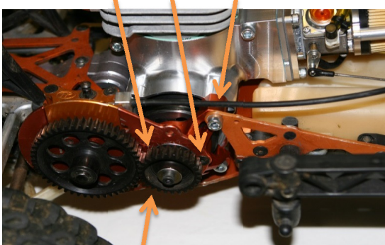
Right side mounting bolts (2 behind pinion)
